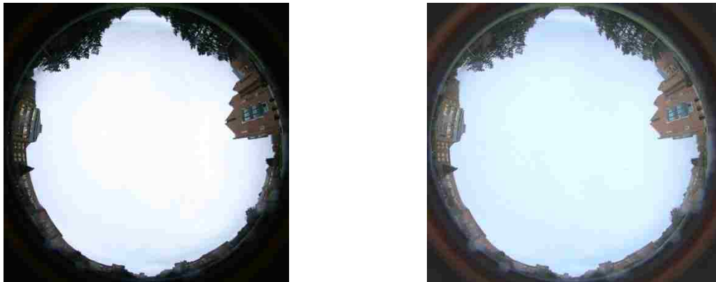
Figure 3 A low dynamic range image (left), and a tone mapped image of a high dynamic photograph (right) of the sky
